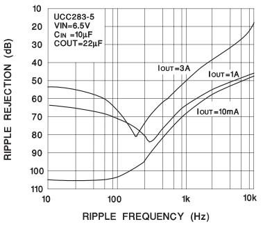
Figure 6. Ripple Rejection vs. Frequency
